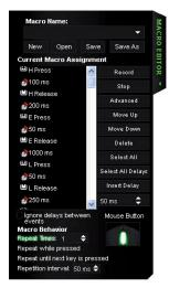
Current Macro Assignment – A list of keystrokes, delays, and other functions that are played back when the macro is executed. As you record a macro, the keyboard keystrokes that you type along with the actual time delays between the events will be listed in the "Current Macro Assignment" window.
